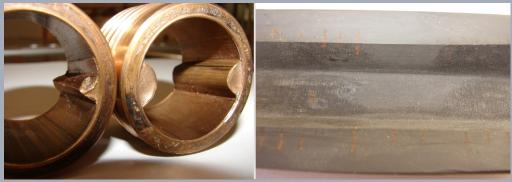
FAST WEARING, INTENSIVE WEARING - UNEFFICIENT PNEUMATIC HAMMER OPERATION
